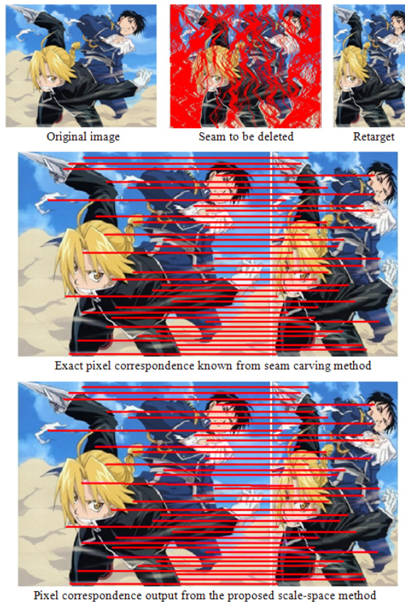
Figure 2: Image retargeting and pixel correspondence. Top row: image retargeting using seam carving method [AS07]. Middle row: exact pixel correspondence between original (392 × 320) and retargeted (196 × 320) images. Bottom row: pixel correspondence output from the proposed scale space method. Only 0.1% correspondence is presented.
