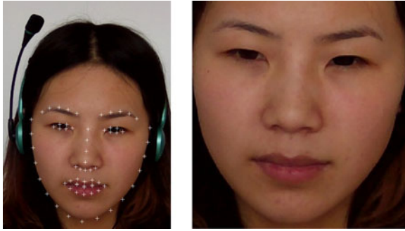
Fig. 1. Left: detection of 66 feature points in a facial region using the DRMF method. Right: the normalized facial area.
