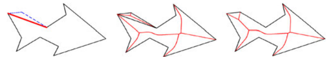
Fig. 19. Two adjacent boundary edges are added outside of the current shape (evolution step 12 in Fig. 18) and medial axes are merged along shared boundary.
