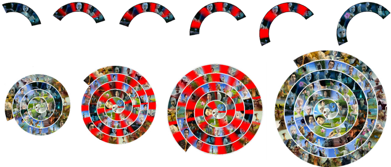
Fig. 4. Continuous zooming in with hierarchical smooth transition. Red areas represent the parts of smooth transition of ROIs in the animated zooming sequence. Top row: local scaling, in which a piece of spiral arc is zooming in from left to right. Bottom row: global scaling, which shows the overall zooming-in of SpiralTape.
