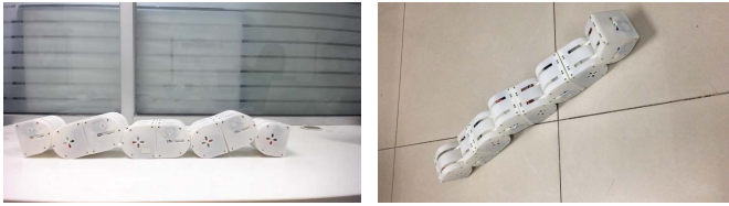
(a) The motion of snake configuration in two scenarios
