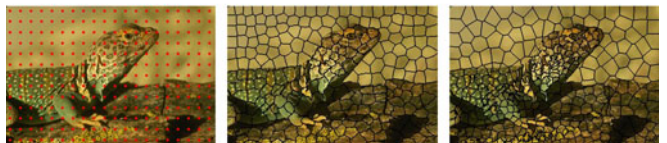
(d) Superpixels by IMSLIC (middle) and MSLIC (right) starting at a uniform initialization on I (left). IMSLIC and MSLIC generate 300 and 366 superpixels respectively.
