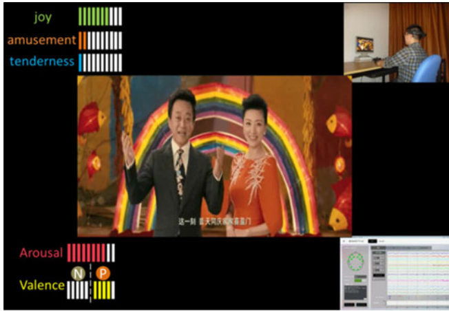
Fig. 5. The human machine interface of the proposed real-time movie-induced emotion recognition system from EEG signals. In this screenshot, our system successfully recognises joy (target emotion) from amusement and tenderness (both are high-arousal and positive emotions).
