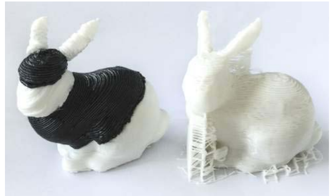
Fig. 1. A bunny model fabricated by our RoboFDM (left) vs. the model made by conventional FDM (right). Note that, to illustrate our decomposition algorithm, different parts of the bunny model being printed along different directions are fabricated by filaments in different colors.
