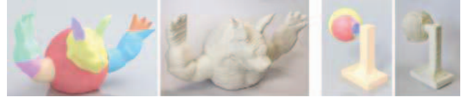
Fig. 8. More examples that are fabricated by our RoboFDM system – (left) Armadillo and (right) Hanging-Ball without adding any supporting structure.
