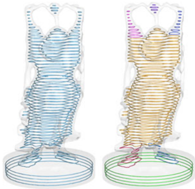
Fig. 7. Contours on the Buddha model (left) are clustered into seven different groups, which are displayed in different colors (right). Contours in each group are connected by strip triangulation to generate an interior surface with simple topology (i.e., genus zero).
