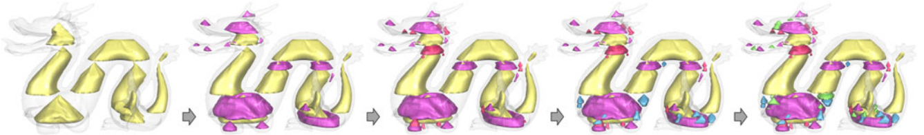
Fig. 12. The volume of a Dragon model can be significantly reduced after repeatedly applying the hollowing operation developed in our framework—inner voids generated in different rounds of hollowing are displayed in different colors. From left to right, the operations result in a volume reduction of 42.9, 57.6, 61.1, 64.9 and 66.6 percent respectively.
