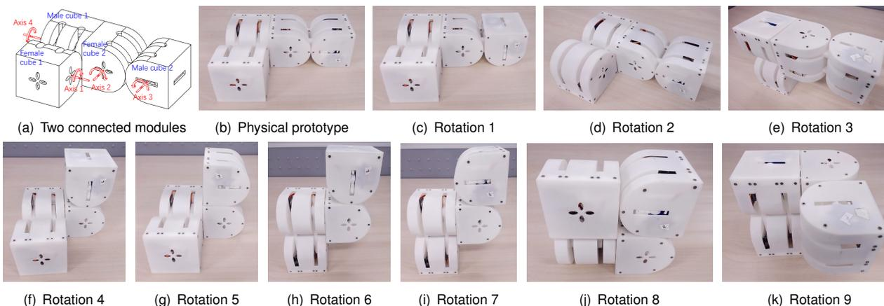
**Figure 1:** Two connected modules can support totally  $3 \times 4 \times 4 = 48$  rotations and nine rotations are illustrated here. More details are in accompanying demo video.
