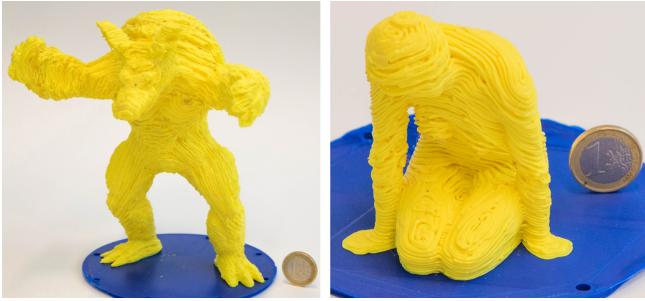
Fig. 10. The results of our algorithm for 3D printing an Armadillo model and a Woman-Pully model by multi-axis motion.
