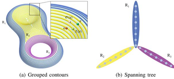
Fig. 5. Spiral paths can be generated from iso-contours of a field  $\mathcal{D}_M$ , and a minimal spanning tree helps to connect the simple set of spirals to cover regions with a complicated topology where each node represents an iso-contour.
