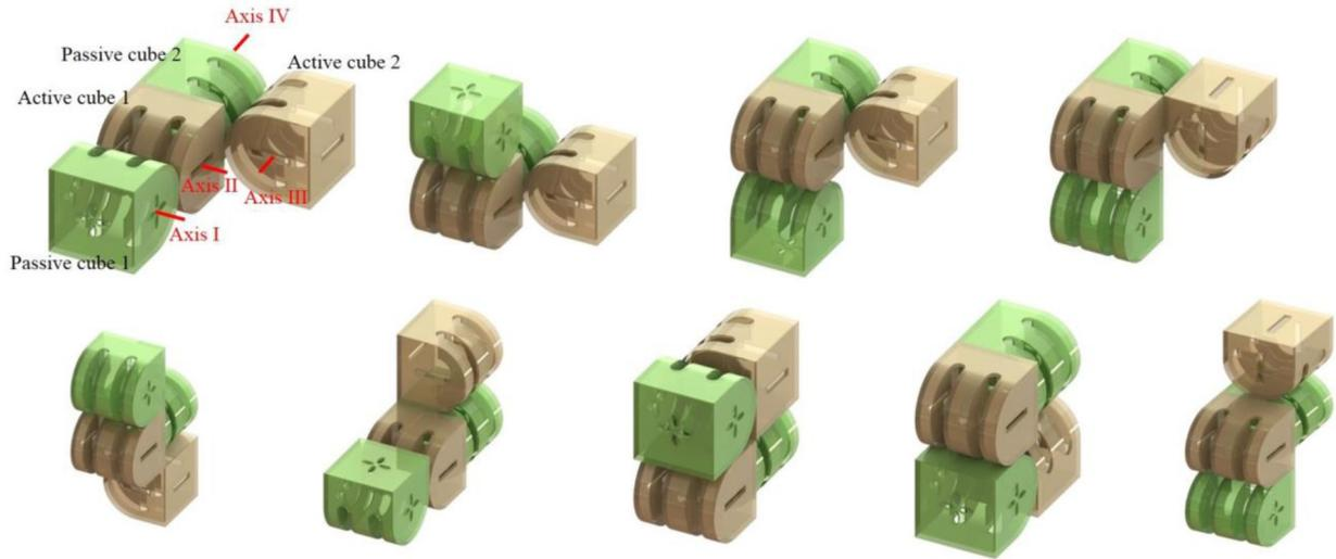
Fig. 3. There are three different ways to connect two EModules. Since each EModule has four rotation DOFs, a total of  $3 \times 4 \times 4$  rotation DOFs can be provided for users to interact with the two EModules. One way to connect the two EModules (top-left) and their nine possible rotations are illustrated in this figure. See accompanying video for more details.
