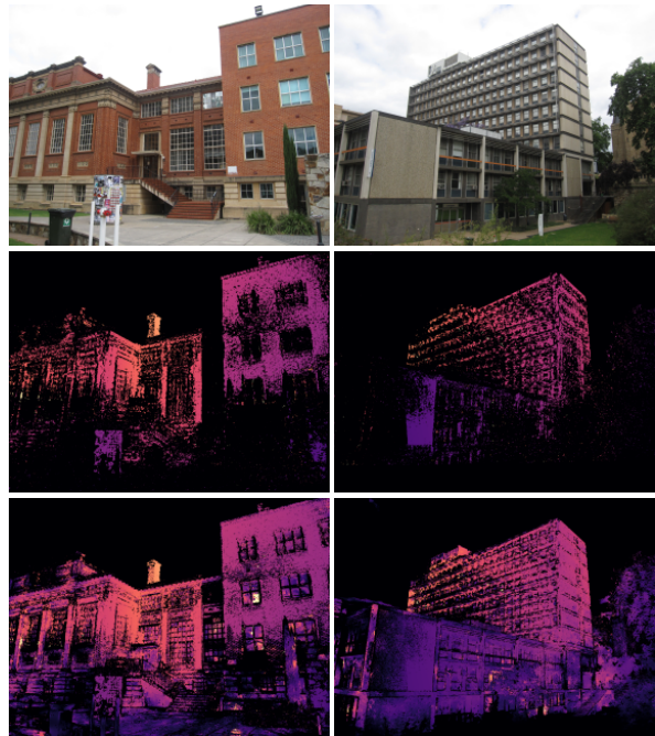
Figure 6. Results on applying the proposed solver over sparse reconstructions from COLMAP [40, 41]. Top row: input image. Middle row: initial sparse depth map acquired from COLMAP. Bottom row: output depth after applying the proposed solver.
