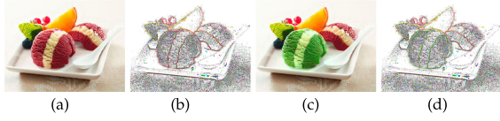
FIGURE 3. Poisson vector graphics guided color editing. The ice cream image (a) is vectorized into a set of DCs (colored, solid lines) and PRs (dotted regions) (b), where the former encodes the low-frequency color and the latter encodes the high-frequency details. To change the ice cream’s color, we only need to edit the boundary colors of the DCs (d). Diffusing the new boundary colors produces an image with a totally new looking (c). Intuitively speaking, we formulate the region-based color editing into a problem of editing the color of its boundary. The only difference between (b) and (d) is the boundary colors of DCs. (a) Original. (b) DCs and PRs. (c) Result. (d) DCs with new boundary colors.
