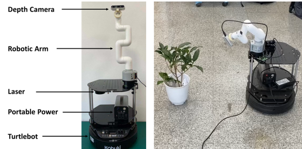
Fig. 1. Our novel designed NBV robot with turtlebot, robotic arm, portable power for powering robotic arm, laser and depth camera as the end effector of robotic arm.
