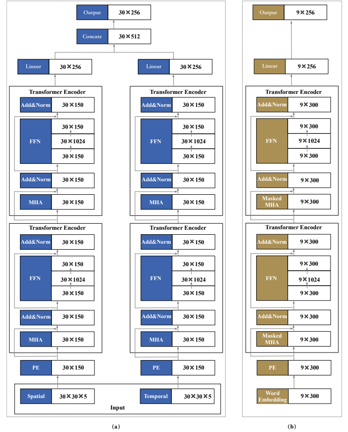
Fig. 4. The structure diagram of spatial-temporal encoding module and label correlation learning module. The left of each block in this diagram is the type of layers and the right is the dimension of its output tensor.
