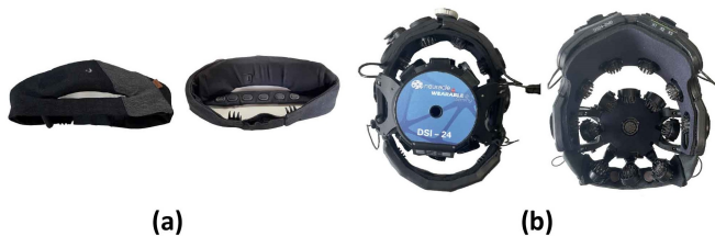
Fig. 5. The snapshots of the devices. (a) 5-channel SleepUp2.0 NaoLubrain EEG device. (b) 18-channel Wearable Sensing's wireless DSI-24 device.
