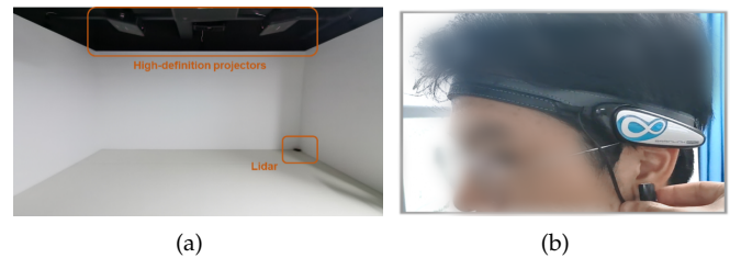
Fig. 5. Some hardware in the prototype system. (a) An immersive CAVE with 4 projectors and 4 Lidars. (b) A low-cost portable EEG headband.
