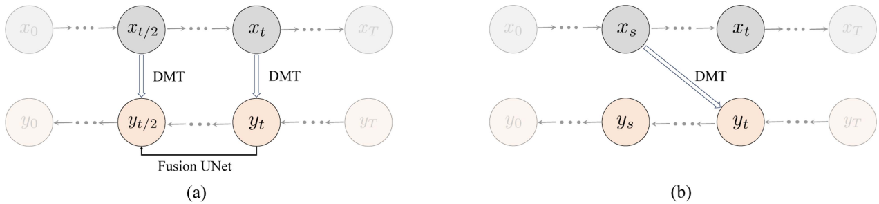
Fig. 4. Conceptual comparison for (a) multi-step DMT and (b) asymmetric DMT. \{x_t\}_{t=0}^T represent different states of the input from the source domain, while y_T \rightarrow y_0 stands for the denoising process of DDPM. Here, T denotes the total number of noise-adding steps in the diffusion process. Multi-step DMT combines the translation results of DMT at two different timesteps with an auxiliary fusion UNet and denoise to achieve the final output, while asymmetric DMT applies translation at different timestep pair (s, t) . More discussions are addressed in Section III-E and Supplementary Material , available online.
