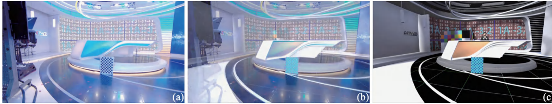
Figure 6 Comparison of co-registered virtual and real frames captured with identical camera and lens parameters. (a) Pure real frame; (b) both real and virtual frames set at 50% transparency; (c) pure virtual frame.
