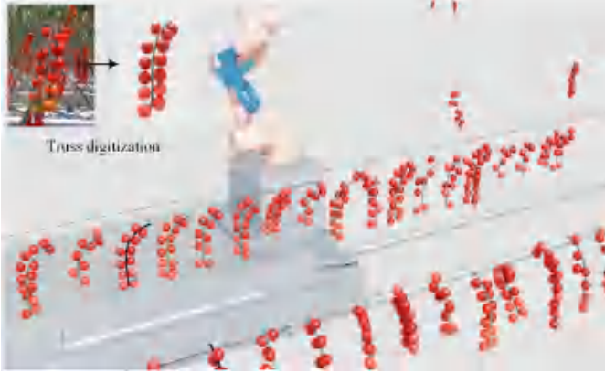
Fig. 12. Built the basic greenhouse structure in Isaac Sim and conducted picking experiments on virtual tomato clusters replicated from real-world scenarios.
