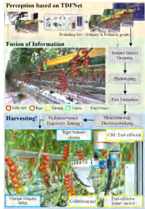
Fig. 1. System overview of the tomato harvesting robot. In the perception stage, a depth camera captures RGB images and depth data from the scene. The TDFNet extracts essential metadata from the RGB images. The fusion stage integrates this information to determine the phenotype parameters and spatial posture of tomato trusses through grouping mechanisms. The harvesting stage employs a decision-making framework to plan a collision-minimizing trajectory and utilizes the proposed circular rotary cutting (CRC) end-effector to accurately sever the peduncle and complete the harvesting process. This integrated system ensures efficient and minimally damage harvesting in real-world environments.
