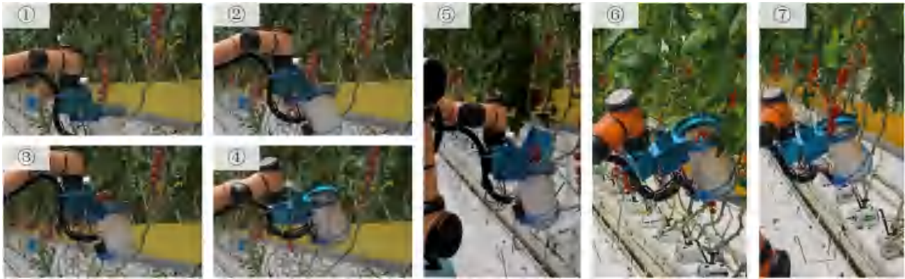
Fig. 14. Examples of harvesting failures. In ①–④, perception errors caused collisions between the harvesting action and the target, leading to displacement. Although the tomato cluster accidentally fell into the end-effector, the robot failed to complete the cutting operation along the designed path. In ⑤, the end-effector collided with the vine in the scene, posing a potential risk of damage if the action proceeded. In ⑥, the peduncle of the target was too long, and due to its flexibility and additional movement allowance, it could not be severed when pressure was applied. In ⑦, the end-effector grazed the vine, causing target displacement. Consequently, the peduncle did not align with the end-effector blade, leading to a cutting failure.
