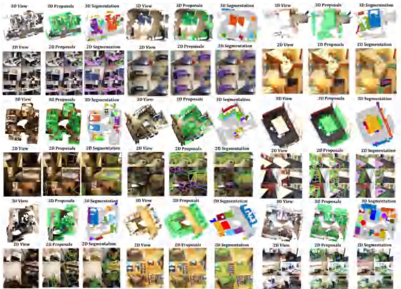
Fig. 13. The WS3D++ corresponding detection and segmentation projections on six rendered 2D views through our proposed multi-view rendering approach. It can be demonstrated that our proposed rendering has established an explicit modality association between the final 2D views and 3D views. Also, by combining 2D and 3D region proposals, more complete and apparent object-level information can be clearly captured both from 2D views and 3D views. Best zoom-in for viewing.
