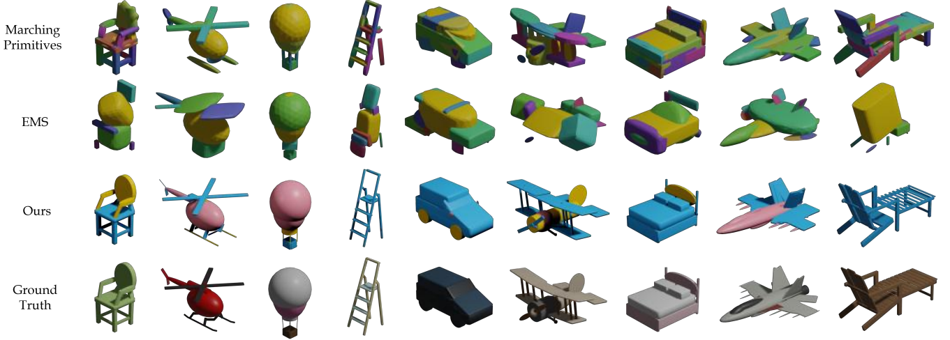
Fig. 4. Qualitative comparisons on the HumanPrim test set: In our method, colors indicate different primitive types, while in Marching Primitives and EMS, colors represent separate superquadrics. Our method achieves human-crafted primitive abstraction and faithfully reproduces the original 3D structure.
